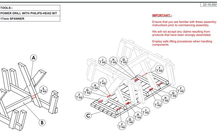
**BEGIN ASSEMBLY WITH THE 2 FRAMES AND** FOOT BRACE SET OUT ON A LEVEL SURFACE.
