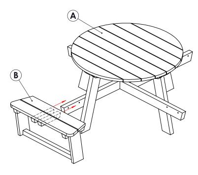
POSITION TIES OF THE PRE-ASSEMBLED SEAT EITHER SIDE OF TABLE'S CROSS-FRAME.
