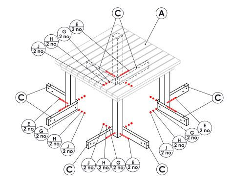
POSITION THE BOTTOM BRACERS AS SHOWN AND FIX M10 x 150mm BOLT THROUGH THE PRE-DRILLED HOLES IN THE LEGS AND BOTTOM BRACERS, ADD WASHER AND NUT AND TIGHTEN UP, COVER NUT WITH BLACK CAP
