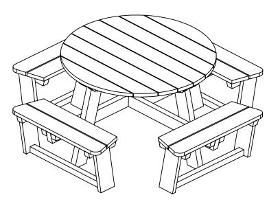
SEAT ASSEMBLY SHOULD NOW BE REPEATED FOR THE REMAINING 3 SEATS, THIS SHOULD FINISH TABLE ASSEMBLY.
