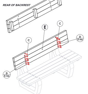
FRAMES, MATCHING THE SEAT ASSEMBLY. FIX THE TOP HOLES WITH 2 x 70mm S/STEEL SCREWS, AND THE **REMAINDER WITH 10 x 90mm S/STEEL SCREWS**
