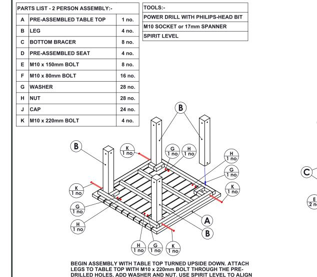
LEGS BEFORE USING M10 SOCKET TO TIGHTEN AND FIX IN PLACE
