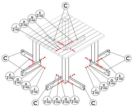
M10 x 150mm BOLT THROUGH THE PRE-DRILLED HOLES IN THE LEGS AND BOTTOM BRACERS, ADD WASHER AND NUT AND TIGHTEN UP, COVER NUT WITH BLACK CAP
