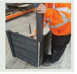
Use the middle post with 3 x dovetail grooves and place onto the 3 panel ends.
