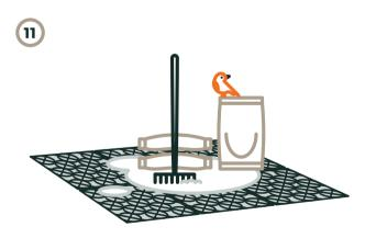
Once all grids are laid, pour on the pea gravel. You should use around 8kg of gravel per individual grid, so for each 3 square metre box of grids you'll need around 216kg of gravel.
