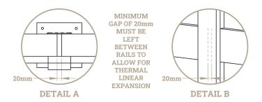
DRILL HOLES SHOULD BE SLIGHTLY OVERSIZED BY 3mm TO ACCEPT SCREWS OR, AS AN ALTERNATIVE INSERT A 10mm SLOT WHICH WILL ALLOW MOVEMENT IN THE FENCING. FULLY TIGHTLEN ALL SCREWS AND THEN BACK TURN SCREWS HALF A TURN ANTI-CLOCKWISE
