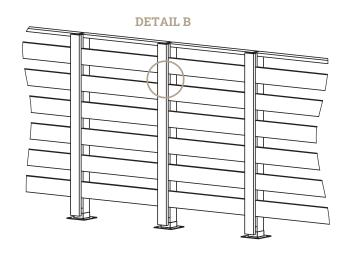
POSTS CAN BE ANCHORED TO THE GROUND USING THE SAME METHOD AS TIMBER AND STEEL POSTS, BY CONCRETING, HAMMERED MECHANICALLY OR SURFACE FIXED.
